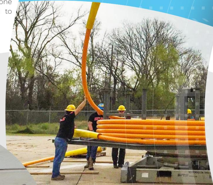
TCP end fittings are simple and reliable and can be re-terminated offshore. The rugged outer coating of the TCP pipe is repairable in offshore conditions. The smooth bore of the pipe with a surface roughness of 5  $\mu\text{m}$  allows for superior flow rates and has an excellent resistance against abrasion. These heavy duty properties ensure a long service life.
