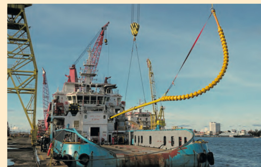
Debutant: Airborne recently delivered to Petronas what it says is the first thermoplastic composite pipe in a full wellstream application Photo: AIRBORNE
