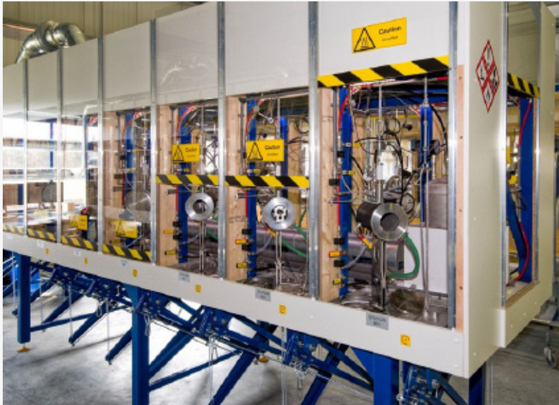
A test frame containing multiple parallel test stations for long-term testing in environment (courtesy of NLR).
