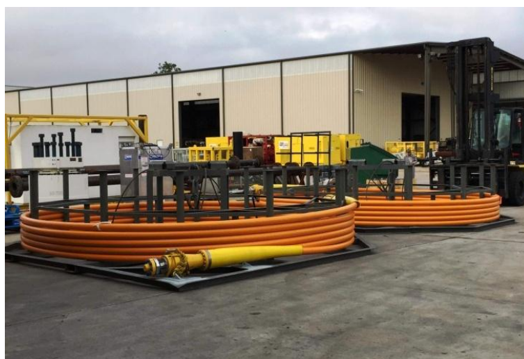
Figure 2 TCP Jumper end-fitting assembly and storage on subsea deployment pallets at local yard
