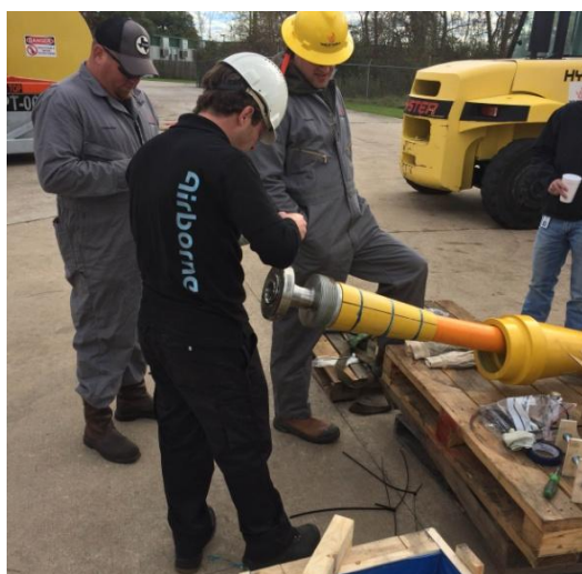
Figure 2 TCP Jumper end-fitting assembly and storage on subsea deployment pallets at local yard
