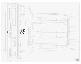
**PIB** Rotate rotary shifter clockwise (01–02–03– ... –18) to position 18 (fig. 20).
