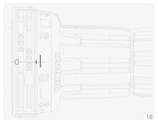
F Switch rotary shifter to position 01 (fig. 18).
