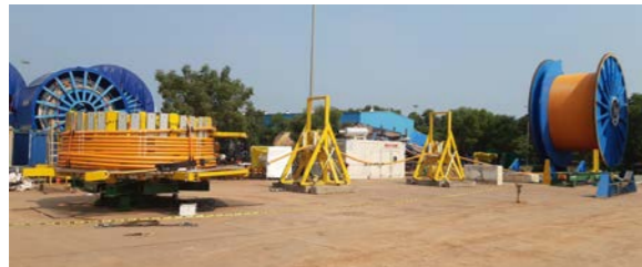
1. Spooling from reel to pallet/reel & cut to required length
