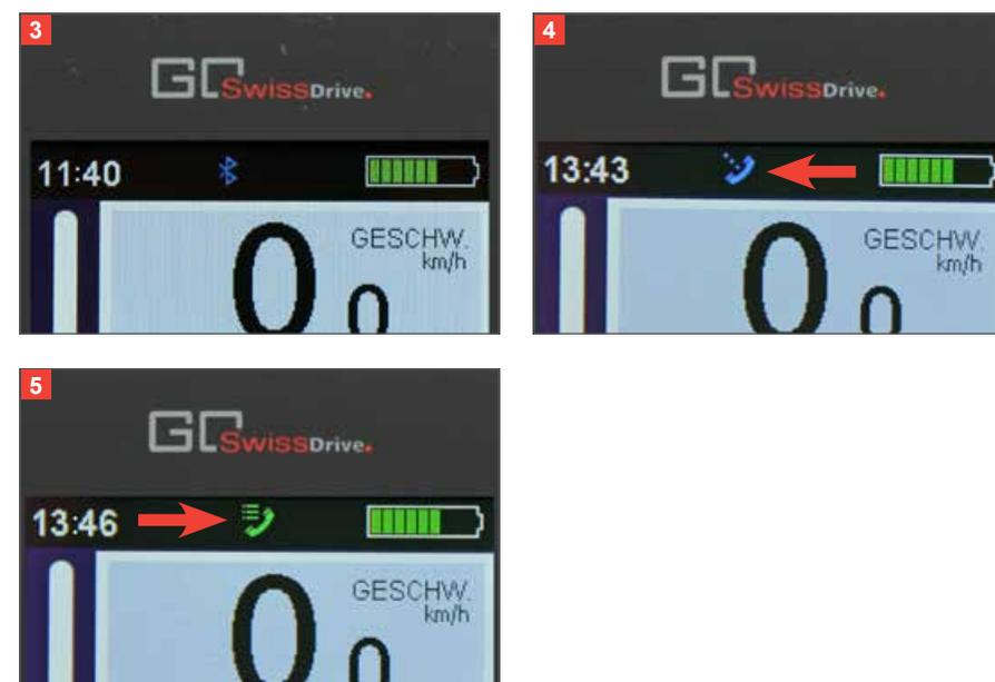
**Service tool (1):** Your well-equipped dealer has the GO SwissDrive service tool. With this tool he can make various settings on your pedelec/e-bike. Once the display is connected via the USB or Bluetooth interface with the service tool, this is visualised by means of the service tool symbol.
