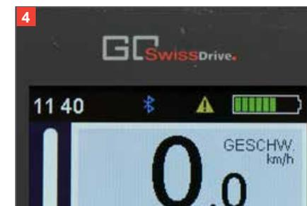
The currently selected **assistance level** is visualized by the graphics on the left edge of the display **(1)**. By means of the +/--keys you can select between five positive assistance levels and two recuperation levels. By pressing the +key you select a higher assistance level, by pressing the -key you select a lower assistance level. By selecting assistance level 0 the motor assistance is turned off.
